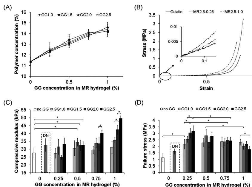
Fig. 3 Polymer concentration of MR hydrogels (A) and mechanical properties of gelatin and MR hydrogels: (B) stress-strain curve (MR $x$ - $y$ : GG concentration is  $x$ % in microgels and  $y$ % in MR hydrogels), (C) compressive modulus and (D) failure strength. Compressive modulus and failure stress of DN hydrogels are added for comparison in (C) and (D) in each dotted box. (\*) Indicates significant difference ( $p < 0.05$ ).
