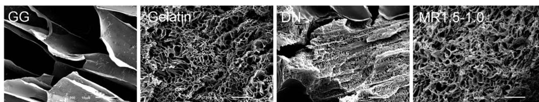
Fig. 4 SEM images of cross-section of hydrogels. The scale bars represent 10  $\mu\text{m}$ .
