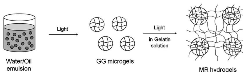
Fig. 1 Preparation procedure of MR hydrogels.
